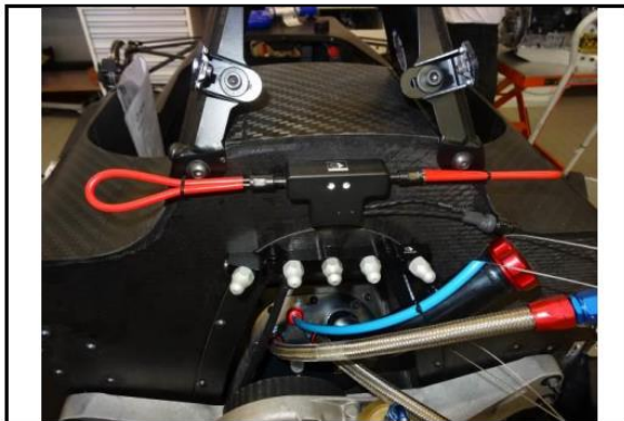
F3-14) Engine compartment spray nozzles + trigger - mounted
