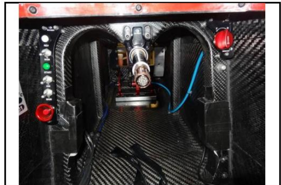
F3-15) Cockpit nozzle + trigger - mounted
